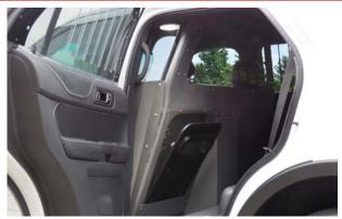
VIPER™ Shield deployed upon releasing T-handle
